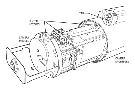
Figure 6. Install Camera Module
